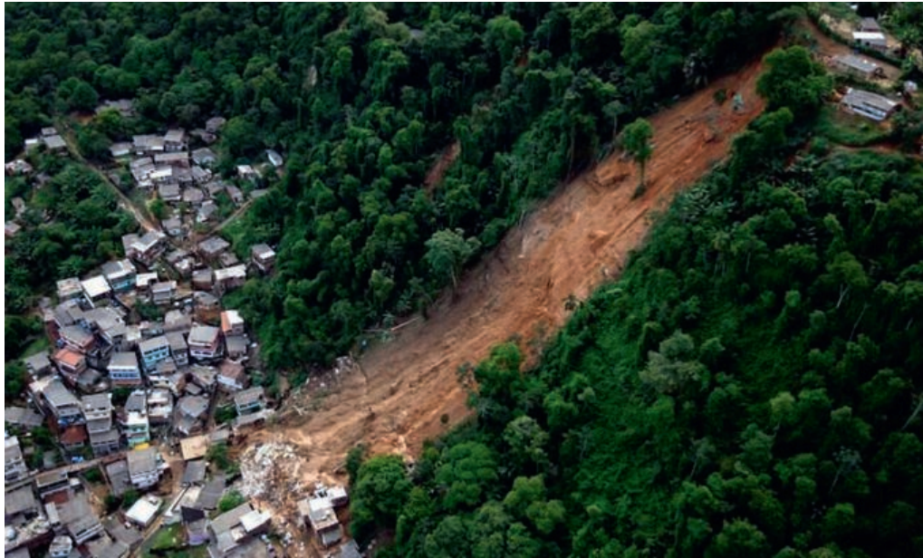
Case Study 8.3 Figure 2 Settlements on hillsides ( bairros-cota ) invaded areas belonging to the Serra do Mar State Park, creating several hazards to its inhabitants, including landslides, floods, road accidents, and freshwater contamination.
