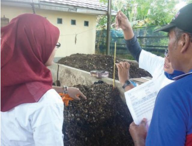
**Case Study 15.3 Figure 4** *Monitoring of the compost temperature at the Material Recovery Facility.*
